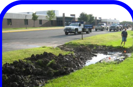
Hand excavated borings indicated there was more permeable granular soil two to three feet below the topsoil.
